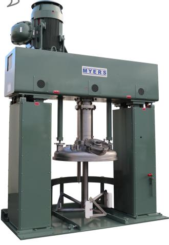
**ABOVE:** 200 HP dual-post, single-shaft reciprocating mixer for highly viscous applications. This mixer is designed to allow two feet of vertical travel of the mixing blade while operating and maintaining the mixing tank at ground level.
